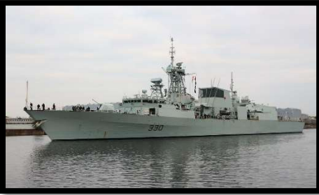
HMCS Halifax antenna array and identification signal on flag hoist
