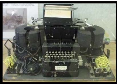
Typex Mk22 cipher machine. (Photo from Jerry Proc via Bletchley Park and Wikipedia)
